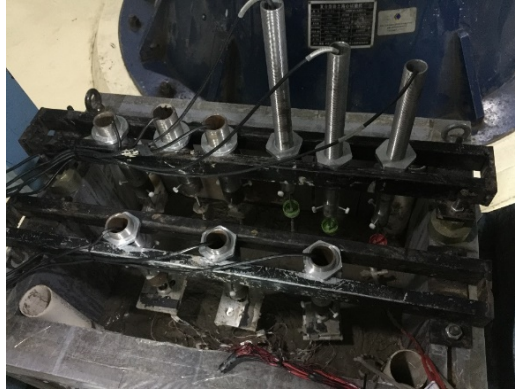
Fig. 3 Pile-soil centrifuge test model
